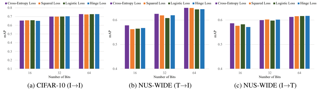
Figure 6.7: The performances of the proposed LPMH with different types of loss functions. The mAP results with different code lengths are reported on CIFAR-10 and NUS-WIDE. ‘I→I’, ‘I→T’ and ‘T→I’ represent “image query image”, “image query text” and “text query image” respectively.
